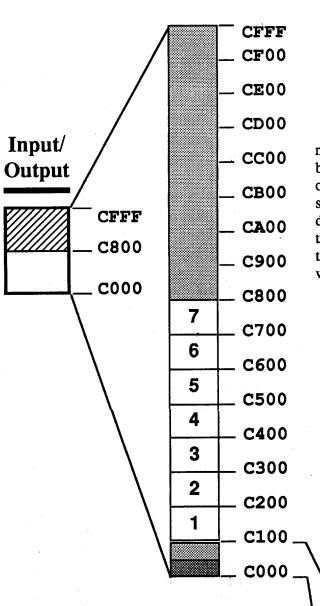
I/O ROM (C800-CFFF) This 2K memory space is supposed to be shared by the cards plugged into the slots on a one-at-a-time basis. Access to the 2K space is gained by first referencing address \$CFFF (to tell all cards to release this space) then any memory access into the Slot ROM of the card needing access will give it exclusive control.
